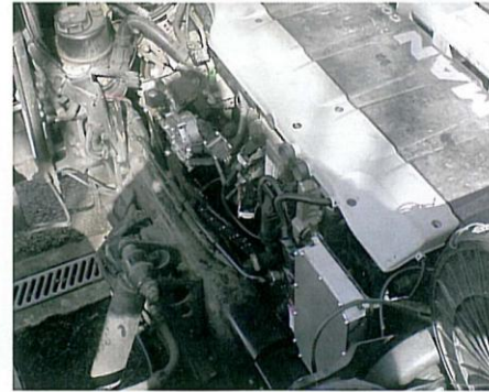
Small change: G-volution Optimiser system in place on MAN D20 engine.
