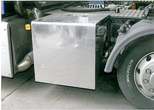
Tactical substitution: LPG tank replaces diesel tank on MAN 6x2 run by R Adams and Sons, with no payload penalty.
